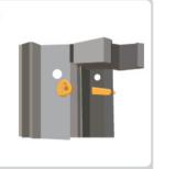
用手搖器把平台調整到適合的工作高度,並用保險銷插入上好安全螺絲帽 Rotate to adjust the platform to a suitable height and locked with the pin to secure in position
